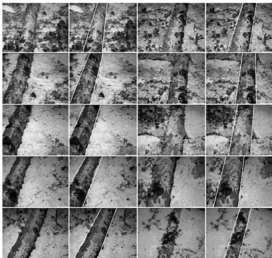
Figure 4: From top to bottom and left to right, tracking results for frames 1-225 of one of the power cable video sequences: (1 st /3 rd columns) original frames; (2 nd /4 th columns) processing results: yellow – cable estimate. (Every 25th frame is shown.)
