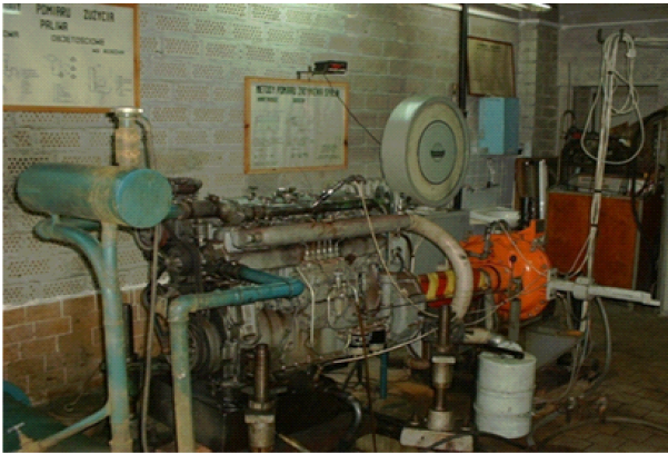
Figure 7: Test stand with 359 type engine
