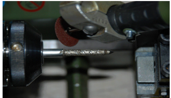
Figure 3: Grinding turbulizing passages on atomizer needle
