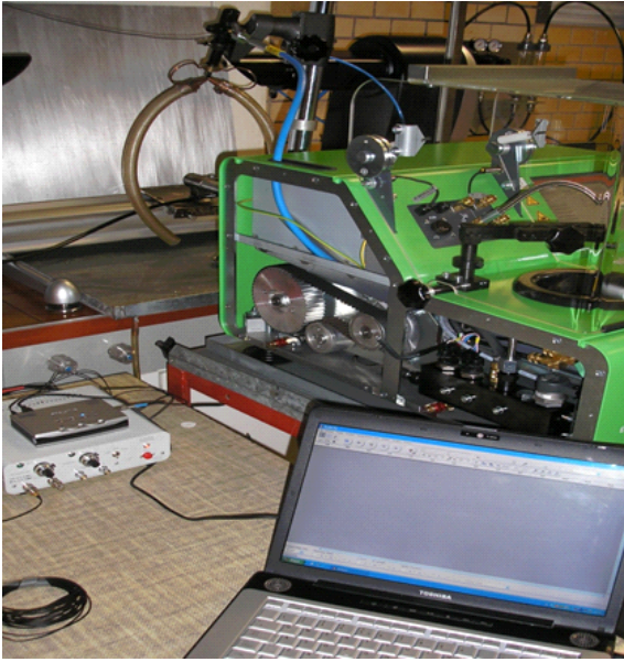
Figure 4: Test stand for particle distribution in atomizer fuel jet
