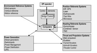
Fig. 1. Schematic diagram of a general DP system, showing the tasks and resources.
