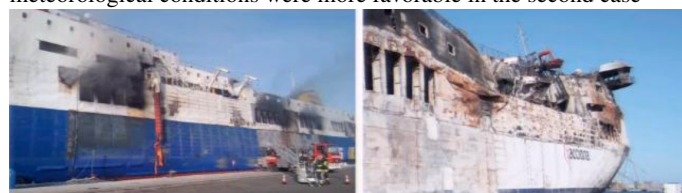
Figure 3: Fire results in the case of "Norman Atlantic" (left) and "Sorrento" (right), where it can be seen that the second suffered far more damage, even though the fire started on the same deck (No. 4) and the meteorological conditions were more favorable in the second case
