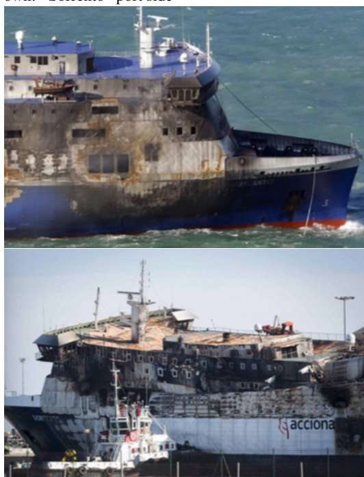
Figure 7: Most affected sides by fire. Up: "Norman Atlantic" starboard side. Down: "Sorrento" port side
