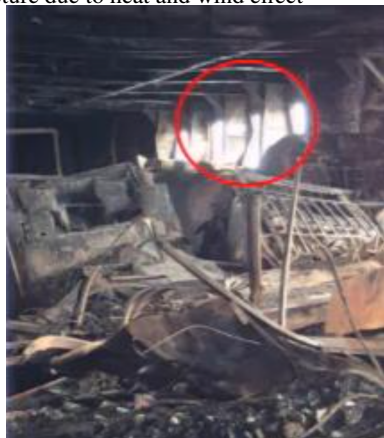
Figure 2: Evidence of major deformation of the "Norman Atlantic" starboard structure due to heat and wind effect
