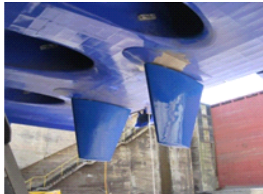
Figure 5: Hanging trimaran rudders to aid navigation.
