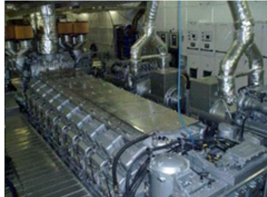
Figure 4: Bow engine room generators.
