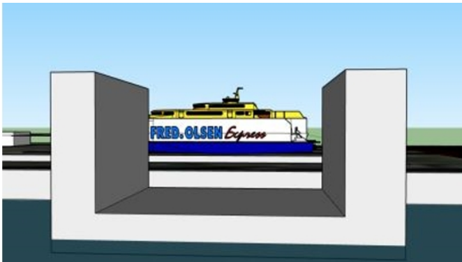
Figure 10: Example of the type of caisson to be used in the dry dock.
