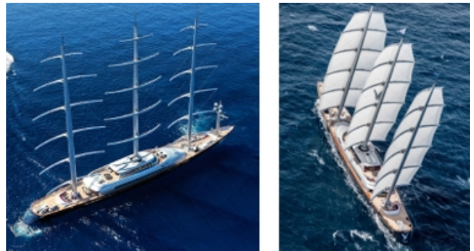
Figure 18: Rotating masts and sails with a concave shape of rails.
