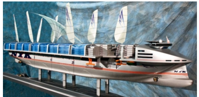
Figure 20: Lids for closing the containers with solar batteries of the NYK ECO Ship 2030.
