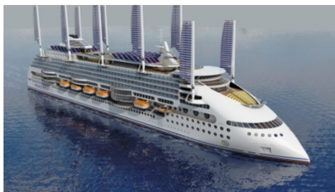
Figure 15: A new concept for placing lifting sails on the roof of ship superstructures.
