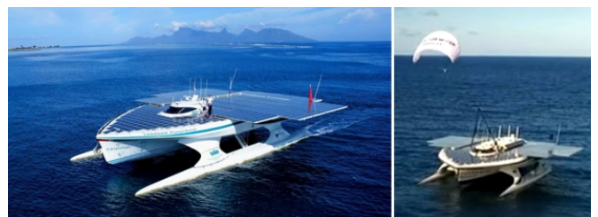
Figure 9: Combination of the "Planet Solar Turanor" yacht (Germany) with a SkySails type sail.
