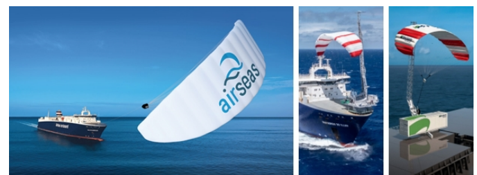
Figure 7: "Airseas" sail system with an autonomous mechanism module for installation on a ship.
