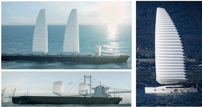
Figure 21: Inflatable mastless sails of the Michelin concern and their descent for passing under bridges.
