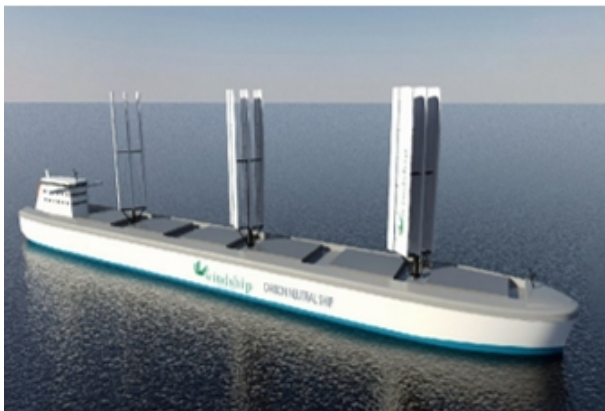
Figure 27: The ASPS hybrid sail propulsion system developed by the Winship consortium.
