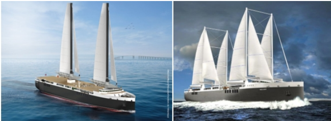
Figure 30: Projects of NEOLINER sailboats with axial and lateral installation of sails.
