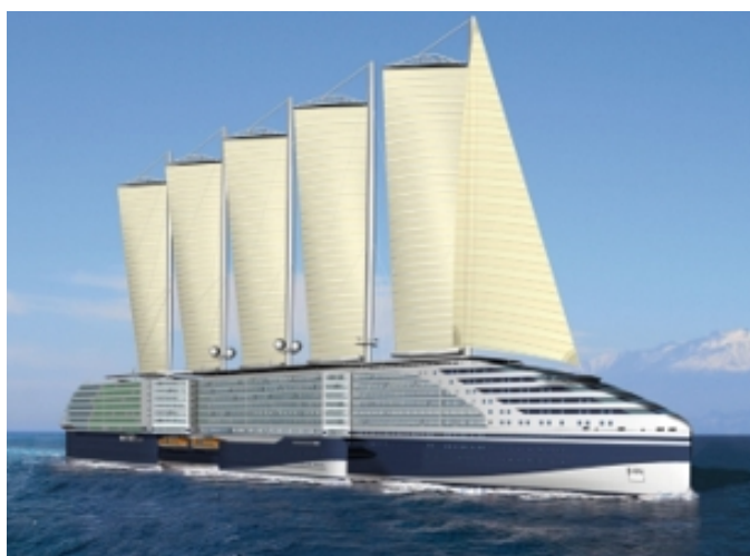
Figure 11: Mast sails in the "Eoseas" passenger ship project of STX Europe (France).
