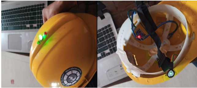
Figure 3: Authors prototype of smart safety helmet.
