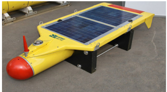
Figure 6: "SANPA" autonomous unmanned solar-powered underwater vehicle (SAUV).
