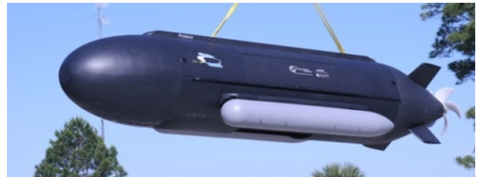
Figure 2: Hydra, an unmanned underwater transportation vessel carrier.
