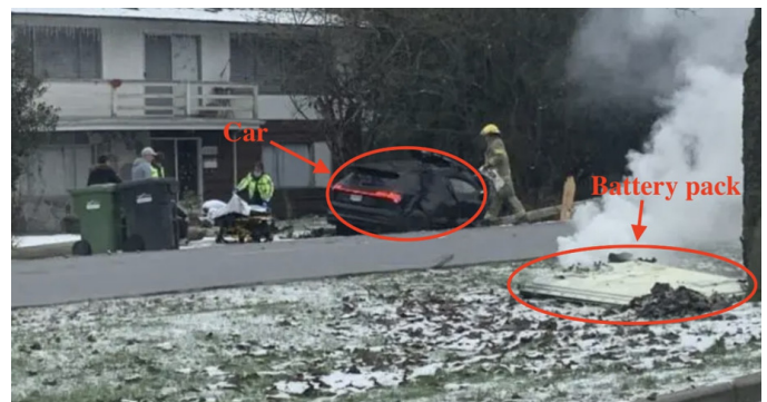
Figure 7: Battery pack of an Audi e-tron is seen being ejected from the EV and onfire.
