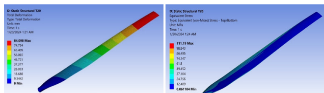
Figure 13: Total deformation and equivalent stress of Epoxy S-glass UD for 20-degree twisted model.
