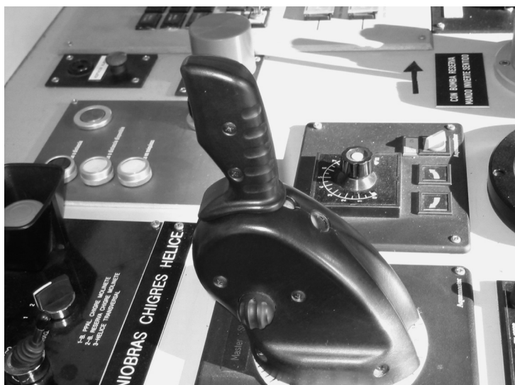
Figure 6. Control Head of one of the two Aquamaster propellers (named Aquamaster Control Head) of the ASD tug "Sertosa Treinta y dos" working-based at La Coruña harbour. To the right of this control, the two push-buttons that constitute the secondary steering system can be appreciated. Photograph: author.
