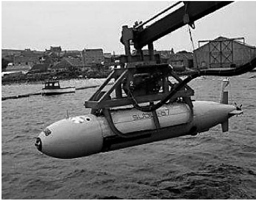
Figure 1a. Geosub AUV ready for trials.
