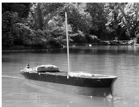
Figure 7: Photo of “Esso Osaka” model during the manoeuvring tests.
