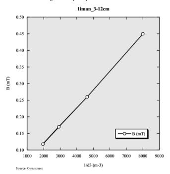
With the greater reliability section, defined between 5 and 10 cm, we proceed to make a new measurement every 1/2 cm and see the variation of the linearity in the sector defined as stable and linear.
