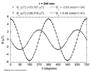
function generates a more homogeneous and lineal, for both sin and cos functions, shown in dashed lines. It is seen that the amplitudes of the field components are not exactly the double one of the other, as they should be according to the equations we handle (6) and (7). Calculating *m* with both expressions, and then calculating its mean value we obtain that  $m = 0.44Am^2$ .
