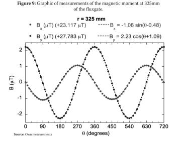
Performing as in previous measurements, adjusted, and finally calculated the mean value, gives us the result that the value of  $m = 0.38 \text{ Am}^2$ .
