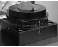
goniometer, where the center of the magnet is placed, and the point of measurement have been placed from the point of measurement of the fluxgate at r distance. We have defined three distances r at what perform such measurements. These will be at distances of 164mm, 244mm and 325mm from the cen-
