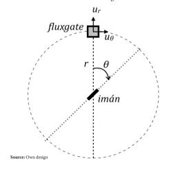
In the approach of the experiment in the preceding figure (Figure 6) we can see the two components B, which are measured by the flux-gate in its x and y axes, for each angle of rotation of the magnet on the goniometer (considering their signs). A specific computer program was generated to collect data generated by the fluxgate.
