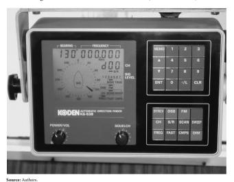
Figure 1: VHF VHF-DF Direction finder (Antenna on cliff).
