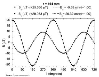
Constant contribution is subtracted in both components. On one hand are represented the values from measurements at different angles of positioning the magnet with a certain symbol, represented by point. Moreover, the adjustment is made that
