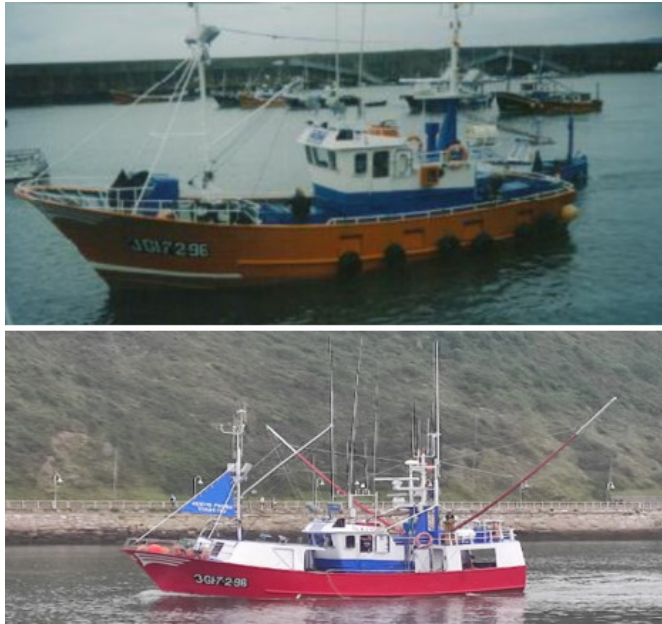
Figure 2: Constructive evolution of fishing vessels, the “Nuevo Padre” boat, an artisanal fishing boat of 16,5 meters in total length dedicated to bottom longline fishing.
