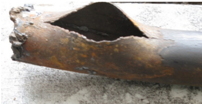
Figure 3: Tube broken through overheating.
