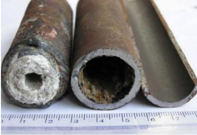
Figure 1: Tubes with internal wall covered with scale.
