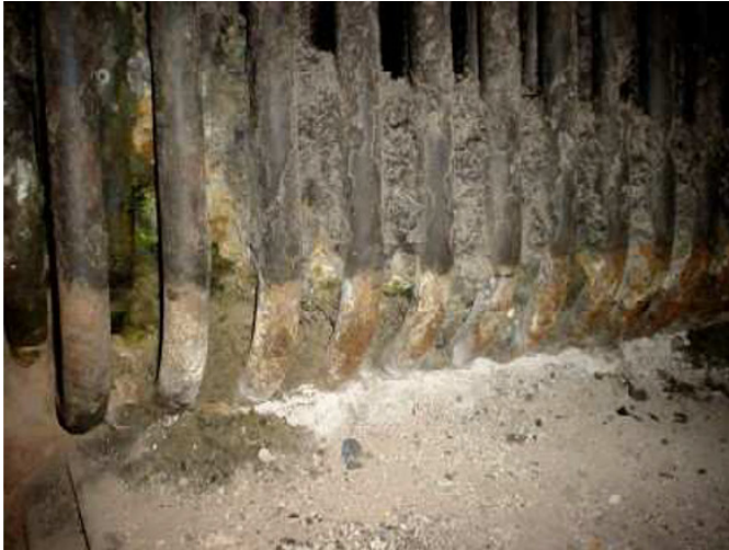
Figure 2: Tubes with external walls covered with soot.
