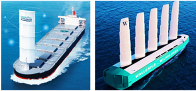
Figure 30: Basic variants of telescopic lifting sails.
