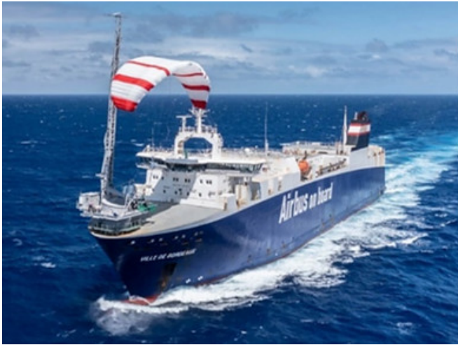
Figure 37: Airseas sail system with an autonomous module of mechanisms for raising and lowering his on the vessel.
