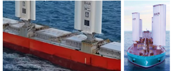
Figure 29: Pedestals with mechanisms on board the vessel for stowing sails on its deck and a variant of doubling the masts by installing them on both sides of the vessel.
