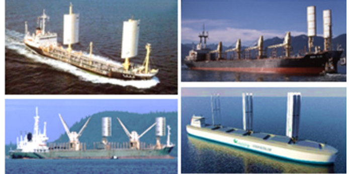
Figure 26: Main projects of ships with rigid sails of the 80-90s of the 20th century.
