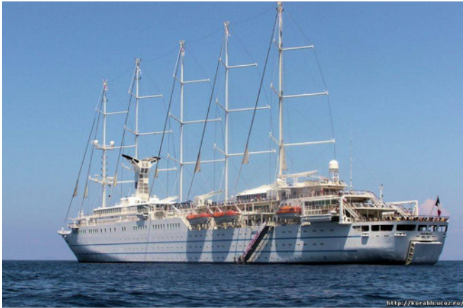
Figure 24: Masts with lateral reinforcing guy wires on the schooner «ClubMed 2».
