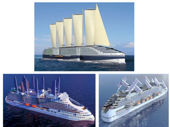
Figure 7: Initial and new projects STX Eoseas project with inclined sails mast along the sides of the vessel.
