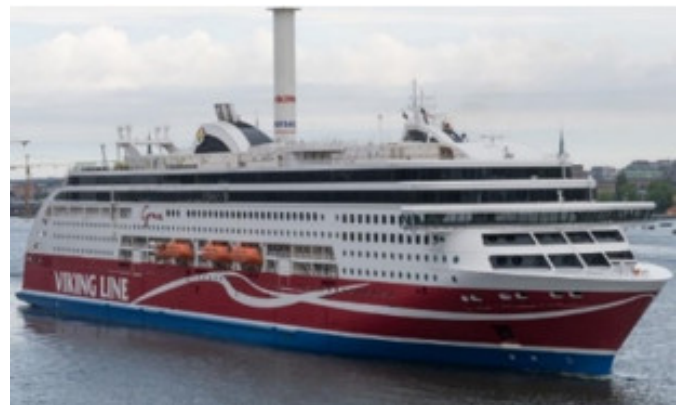
Figure 33: Rotor column on the roof of the M/S Viking Grace cruise ferry.
