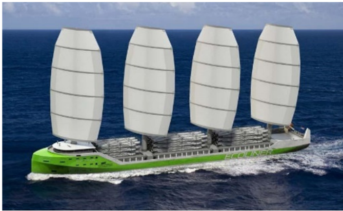
Figure 12: Development of the B-9 project based on the designs of the pleasure yacht Maltese Falcon.
