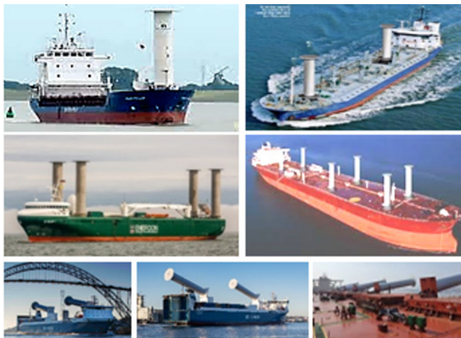
Figure 5: Real ship wind systems with Fletcher rotors and their inclination.
