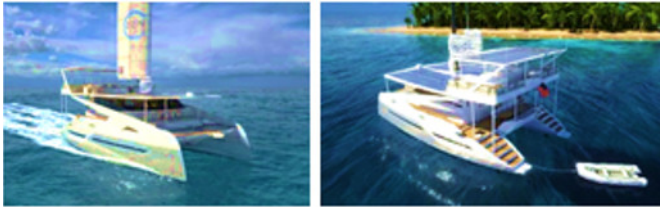
Figure 21: Hybrid catamaran yacht with automatic flexible mast sail and solar panels.
