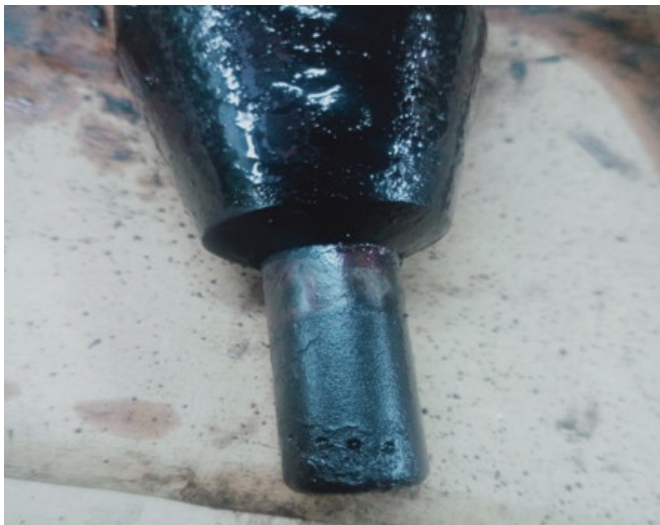
Figure 1: Encrustation at the nozzle tip.
