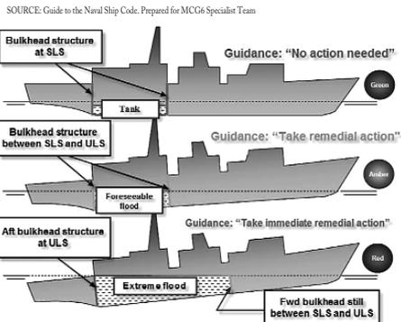
Figure 4. Structural Limit State Zones.
