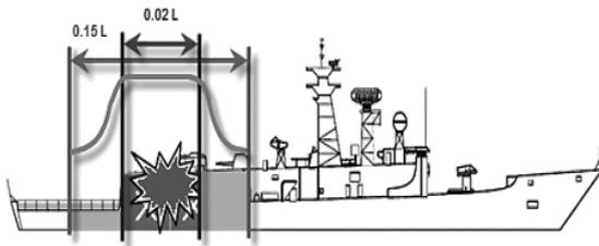
Figure 3. Damage extent on naval ship profile.
