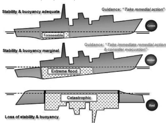
Figure 5. Severity of Damage Event for Stability
