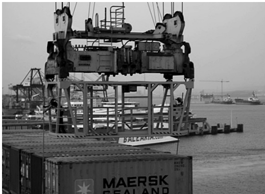
Figure 1. Detail of stevedore unlashing containers at height from a safety cage.
