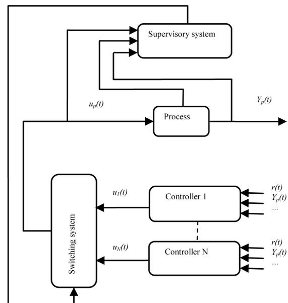
Figure 1. Multi-controller structure.
