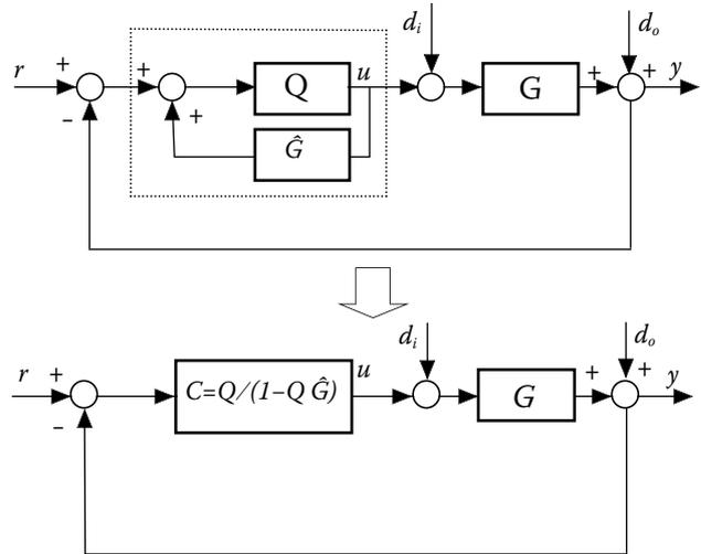
Figure 5. Classical Feedback Control Structure.
