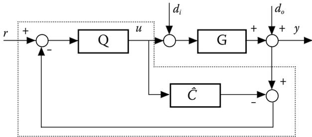
Figure 4. Internal Model Control System structure.
