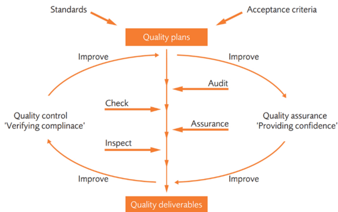
Figure 2: A Typical Quality Assurance and Control System.
