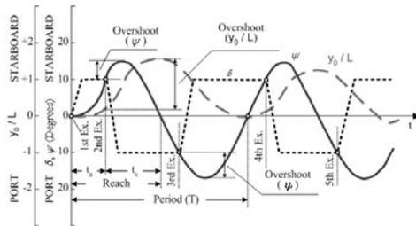
Figure 4: Zig-zag manoeuvre graph: rudder angle  $\delta$ ,  $\psi$  ship's course,  $y_0/L$  normal distance to the initial trajectory divided by the ship's length.
