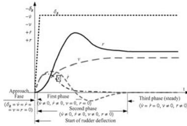
Figure 2: Characteristics of phases of a turning circle.
