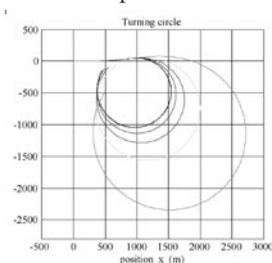
Figure 10: Turning circle for various rudder angles  $\delta$ .
