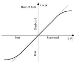
Figure 5: Graph of direct spiral manoeuvre of a stable, symmetrical vessel.
