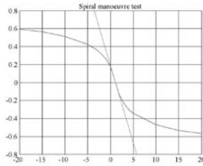
Figure 12: Graph with results of spiral test 20°/20°.
