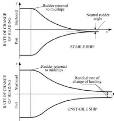
Figure 3: Presentation of results of the Pull-out manoeuvre.
