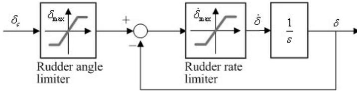
Figure 7: Simplified Diagram of the rudder control loop.
