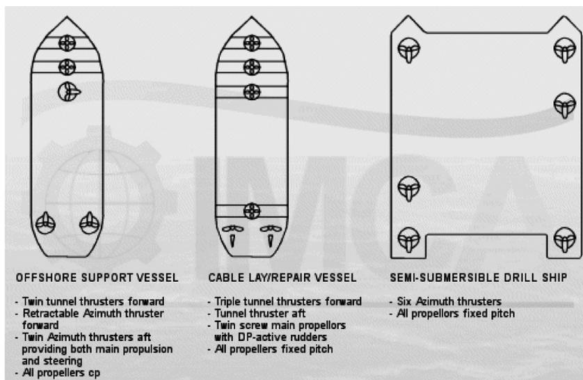
Fig. 8. Typical Propulsion System Layouts.
