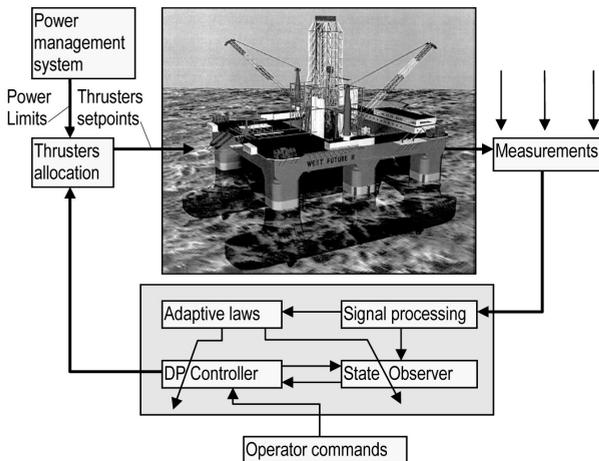
Fig. 2. The general arrangement of a DP system.
