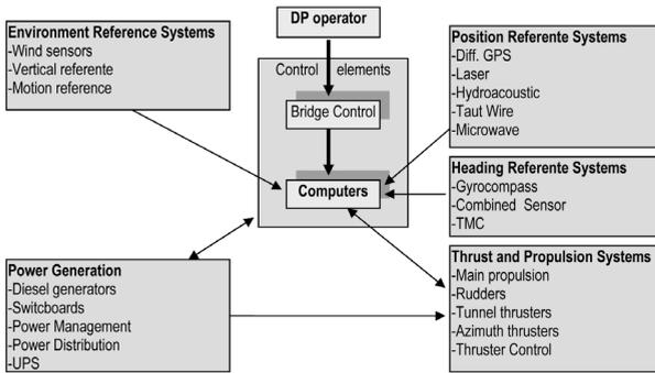
Fig. 1. Schematic diagram of a general DP system, showing the tasks and resources.
