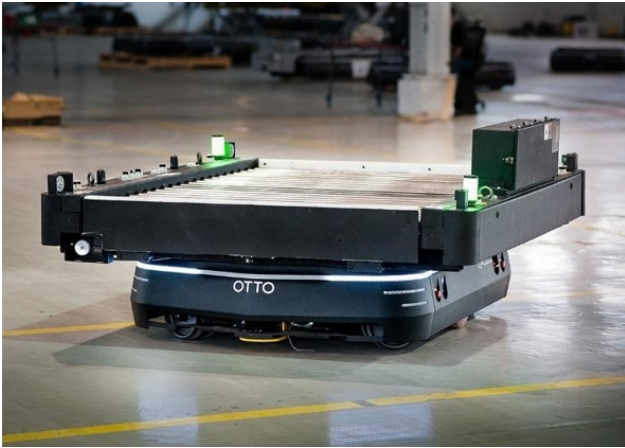
Figure 3: OTTO 1500 can be equipped with a conveyer belt.
