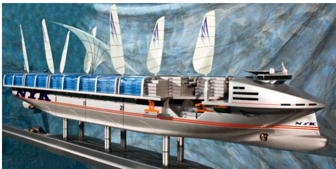
Figure 10: Main view of NYK ECO Ship 2030 container ship with lifting sails and container covers that are equipped with solar panels [20] (Japan).
