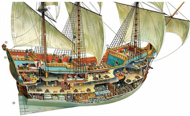
Figure 4: Spanish galleon of about 1,000 tons and two decks during the 16th century, distribution of spaces.
