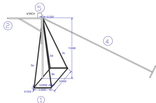
Figure 2: Schematic of the adjustable length support bar (fig-1(4)).
