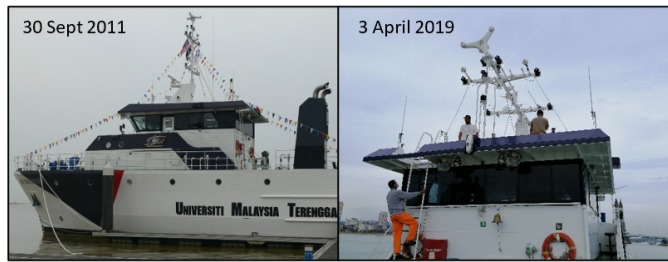
Figure 5: RV Discovery with original fixed mast in 2011 (left) and collapsible mast in 2019 (right).
