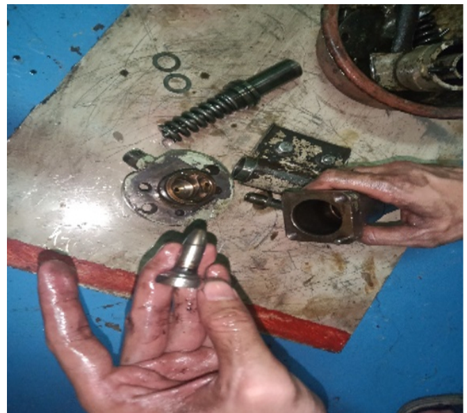
Figure 4: Disassembly of the injector.
