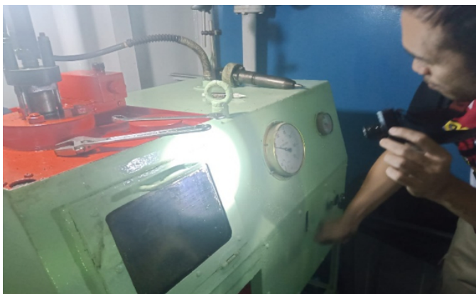
Figure 3: Injector Pressure Test.
