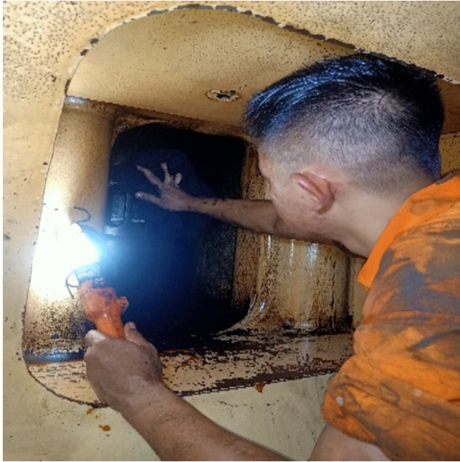
Figure 5: Cleaning the scavenging air chamber of cylinder no.2 on main engine.
