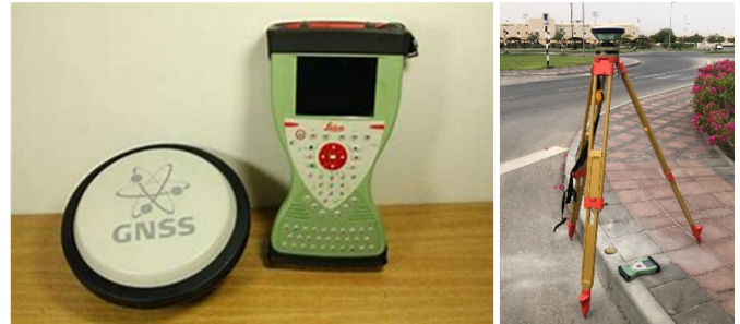
Figure 5: Leica GS14 and CS15 and the Field Survey set up.
