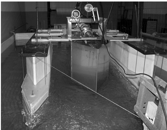
Figure 7. Bollard pull trial under real conditions (fixed pull point).
