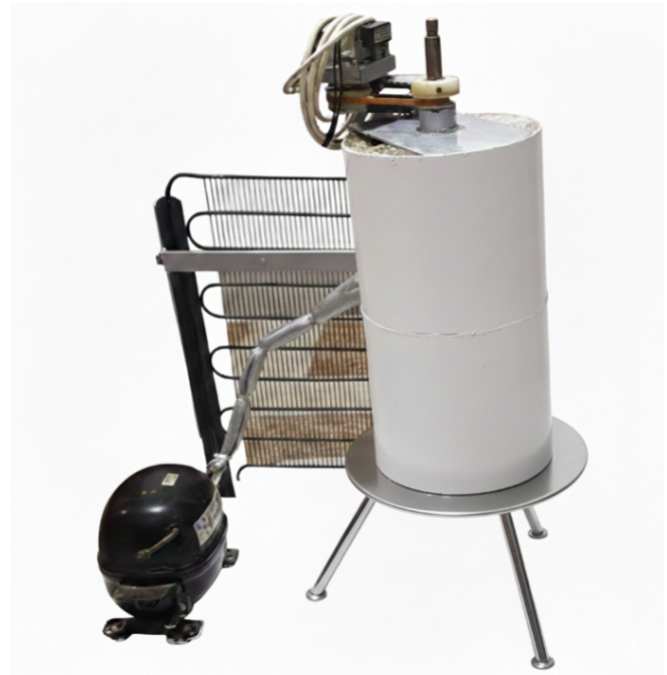
Figure 3: Actual flake Ice Maker Prototype.
