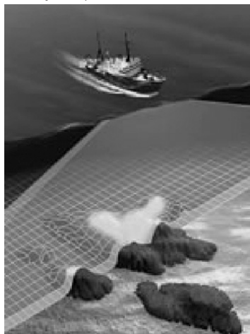
Figure 1. Image of a multibeam echo sounder scanning (Hydroacoustics).
