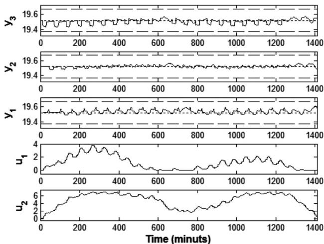
Figure 9: Evolution of Outputs (with seaworthiness bounds) in meters respect to the mean sea level and inputs in  $m^3/s$  in a 24 hours hypothetical scenario
