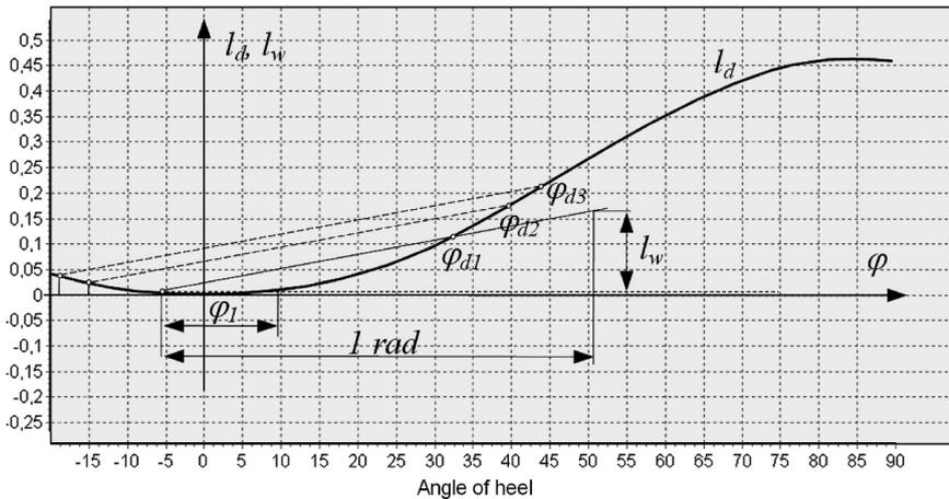
Fig.5. Determination of dynamic angles of heel for ship of 888 project type – for  $Z_v=6.46$  m.
