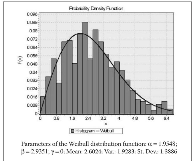
Figure 5. Corrosion depth [mm] measured over the bulk carriers being in exploitation 25 years (cargo: iron ore).
