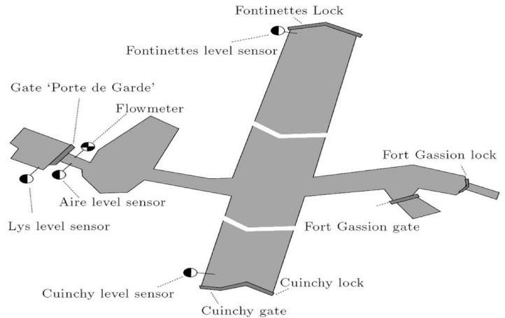
Figure 2: Scheme of the Cuinchy-Fontinettes navigation channel.
