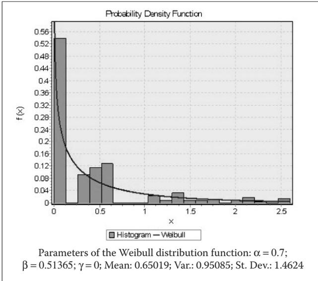
Figure 2. Corrosion depth [mm] measured over the bulk carriers being in exploitation 15 years (cargo: grain).
