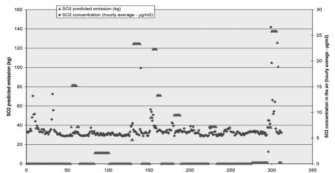
Figure 4: – SO<sub>2</sub> predicted emission and concentration in the air.
