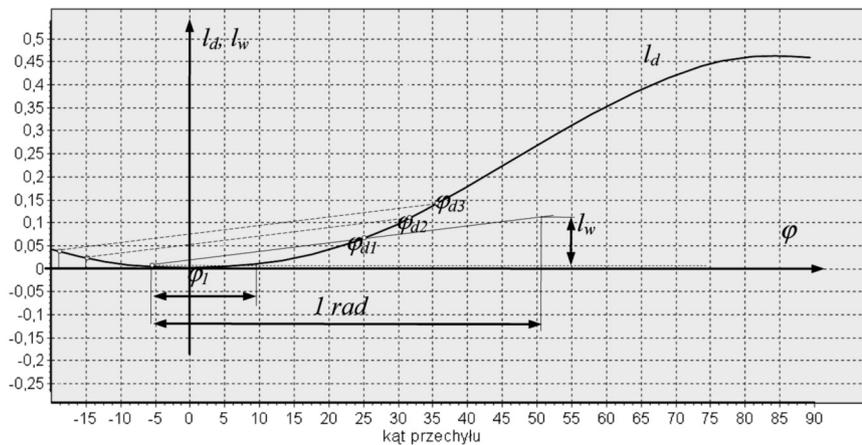
Fig.6. Determination of dynamic angles of heel for ship of 888 project type – for  $Z_v=4.49$  m.
