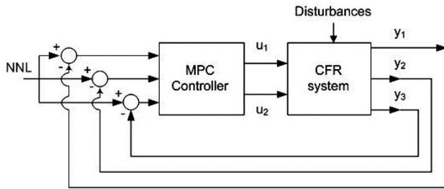
Figure 7: Automatic control scheme.
