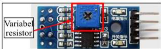
Figure 3: Rearview of the TCRT-5000 sensor.
