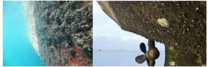
Figure 2: Condition of the outer shell of the ship’s hull.
