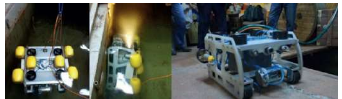
Figure 9: The developed ROV device for the remote inspection and laser cleaning of ship hulls.
