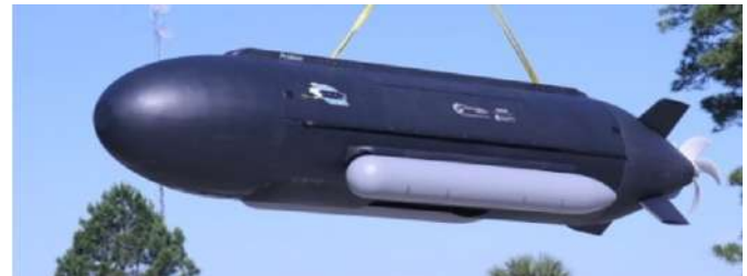
Figure 2: Hydra, an unmanned underwater transportation vessel carrier.
