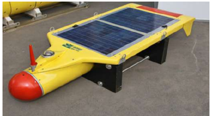
Figure 6: "SANPA" autonomous unmanned solar-powered underwater vehicle (SAUV).
