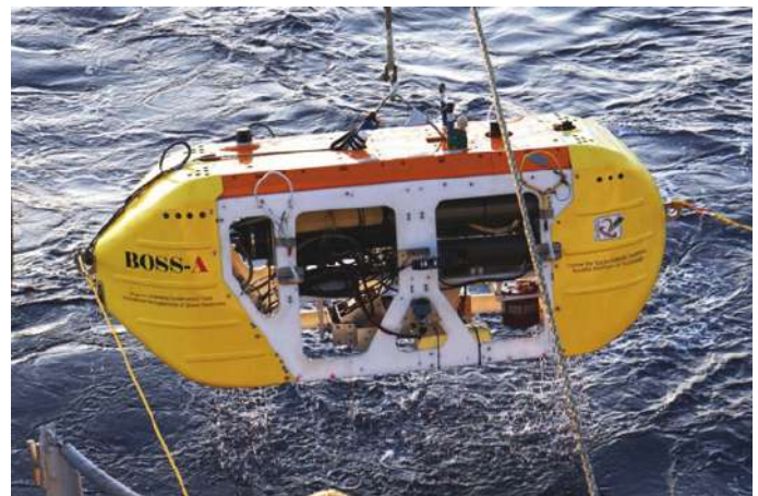
Figure 9: AUVBOSS-A with a visual-acoustic device for inspection of manganese crusts located at 1,000 to 2,400 m depths.
