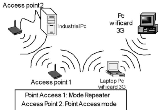
Figure 4. Elements which make up the wireless network
