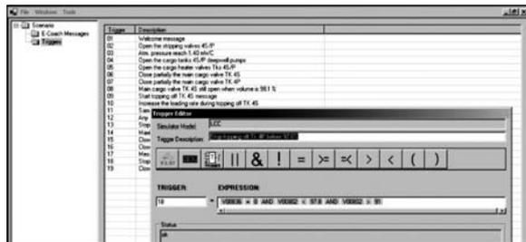
Figure 5. Example of triggers for Topping off exercise.
