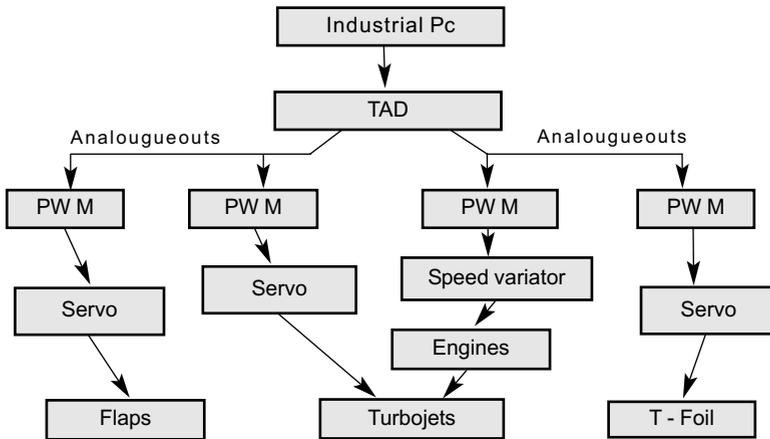
Figure 3. Control of propulsion.
