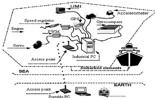
Figure 2. Elements necessary for the monitoring of a trajectory.
