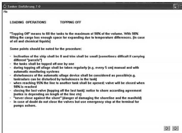
Figure 2. Example of LMS theory module for Topping Off one tank.
