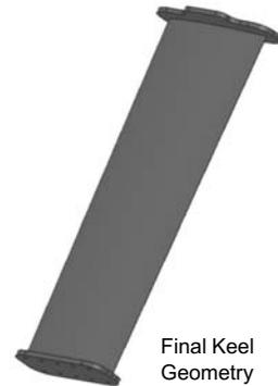
With this optimization we have developed a section with a lower drag and better lifting potential than the baseline. The blade is also lighter therefore we can make the bulb bigger also. The only drawback is the reduction on safety factor. This comes to be expected as we have reduced quite a bit the amount of supporting material in the keel. However, the righting moment has increased considerably.
