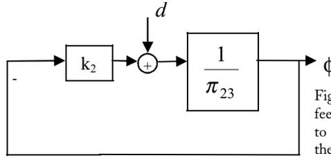
Fig. 4. The SISO feedback system to be solved in the design of  $k_2$ .
